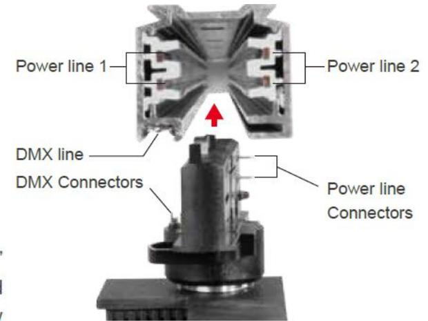
The Track System Kessil offers is an architectural grade surface mounted track consisting of seven conductors allowing for two unique power circuits. Each track features a 22 gauge nickel plated copper Data Bus providing **DMX control signals** to any connected fixture along the track.
